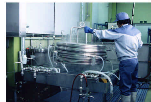
温超純水 & 超音波洗浄 Warm Ultra Pure Water and Ultra Sonic Cleaning
