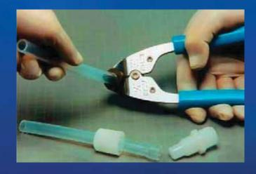
Using the manual flaring method is the fastest, easiest installation system available today, taking just 10 to 20 seconds to install a tube-to-fitting connection using a simple hand tool. No heating or preparation is necessary. This simple method alone can save up to 70 percent of the installation cost.
